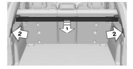
Pull out the cargo cover, arrow 1, and hook both sides onto the brackets, arrow 2.
