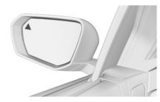
The warning light in the exterior mirror warns of a possible collision.
