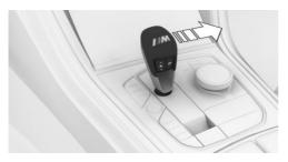
Push the selector lever out of the center position in the D/S direction.
