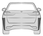
The radar sensors are located on the side in the rear bumper.
