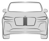
The front camera is located in the radiator grille.
