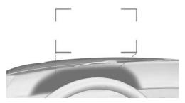
Head-up display views are projected onto the windshield using protective glass. The protective glass is located between the steering wheel and windshield.
