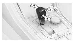
Push the selector lever out of Drive mode in the D/S direction, arrow 1, or shift via the selector lever, arrows at 2.
