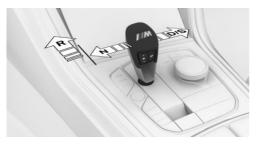
With the driver's seat belt fastened, press on the brake pedal and pull or push the selector lever in the required direction. The selector lever automatically returns to the center position when released.
